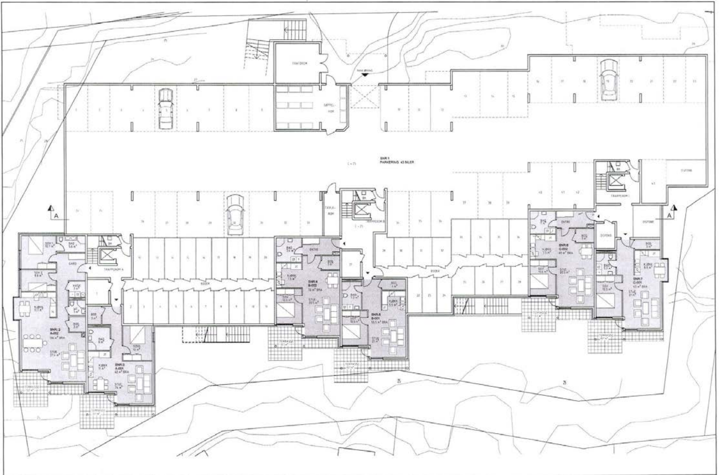
Plan u.etg / parkeringsanlegg.
